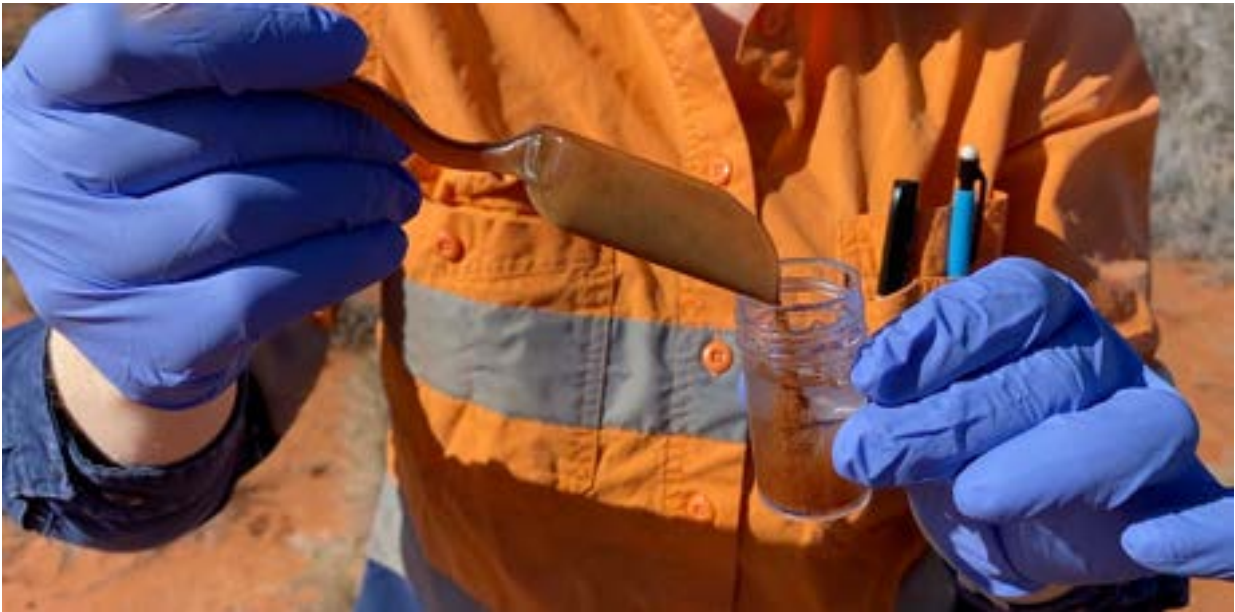
Figure 6.2 Soil samples being preserved in Lifeguard preservation buffer at Roxby Downs.
